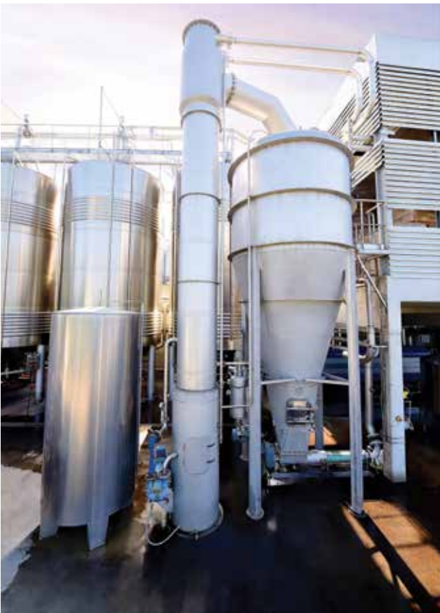
20 t/h vacuum chamber with condenser
