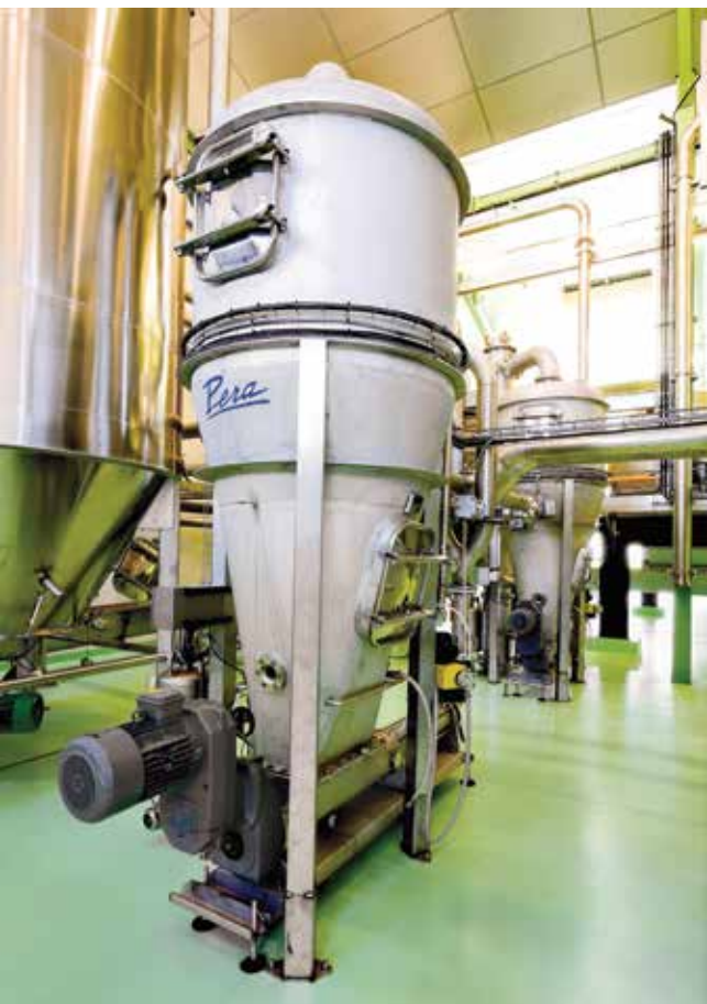
Vacuum chamber 7 t/h, with condenser
