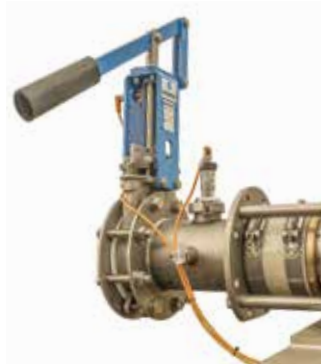
Axial feeding with manual valve
