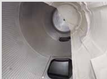
Interior of a pierced tank with membrane and pomace recentring coils
