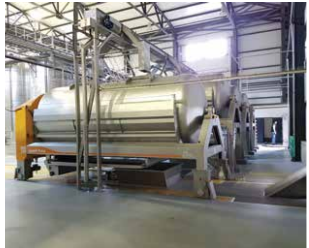
Pomace evacuation by endless screw
