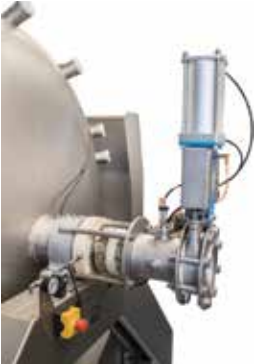
Axial feeding with pneumatic valve
