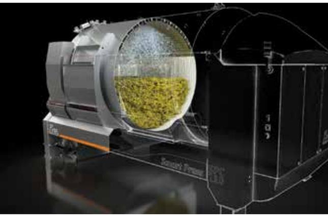
*Injection of anti-oxidant during the crumbling phases*
