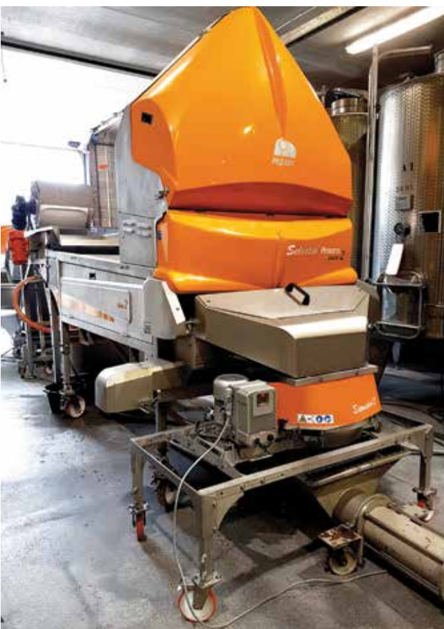
Extractiv' 2 on roller leg chassis at outlet of Selectiv' Process Vision 2
